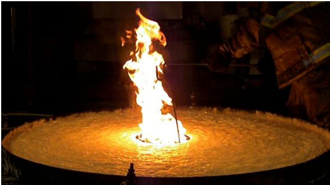
Figure 1: Firefighter placing the started pan in the foam-covered fuel at the beginning of the burnback test
