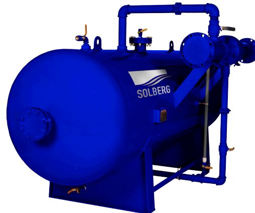
with a with a nylon reinforced neoprene rubber bladder. It has a perforated center tube, and a .37" (9 mm) water channel between the water inlet and water drain valve, which creates a water path between the bladder and tank shell. Openings that are greater than 1.0" (25 mm) will be divided to prevent bladder damage.
