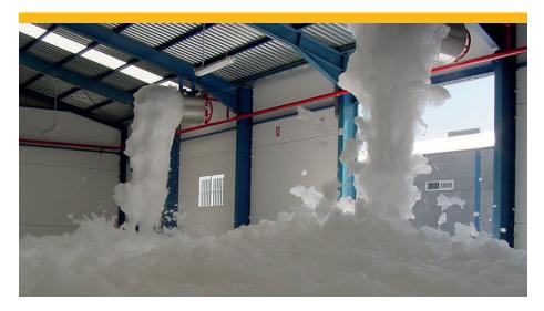
when it is necessary to extinguish light hydrocarbon fires use gentle application and increase the application rate (I/min.m2) (note that in these cases an AFFF com-pound is more efficient).
