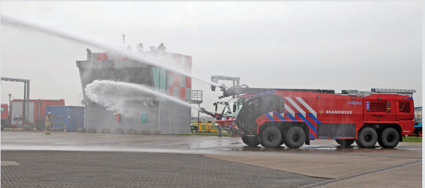
Perimeter Solutions technical personnel went onsite to Schiphol Airport and worked with ARFF truck manufacturer OSHKOSH and airport personnel to test SOLBERG RE-HEALING RF-3 in existing equipment.
