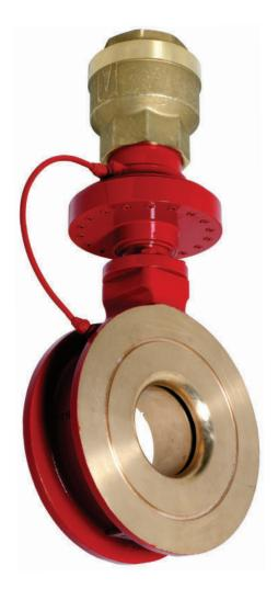
The SOLBERG Foam Pump Proportioner is manufactured using a bronze body and bronze pressure balancing valve for corrosion resistance. The SOLBERG Foam Pump Proportioner is to be installed with a minimum of 5 pipe diameters (30.0" (762 mm)) of straight pipe both upstream and downstream of the proportioner. The proportioner body is cast with a directional flow arrow on the proportioner body indicating the proper orientation of installation.
