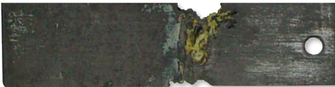
Magnesium exposed to a non-approved product.
